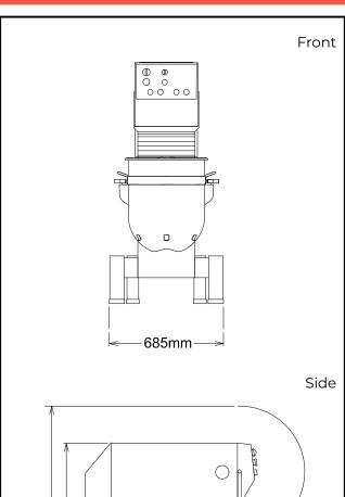
Electric 380-440 V/3N ph/50/60 Hz Supply voltage: **Electrical power max:** 4 kW **Total Watts:** 4 kW Capacity: Performance (up to): 25 kg/Cycle Capacity: 80 litres Key Information: External dimensions, 685 mm Width: External dimensions, Depth: 1050 mm External dimensions, 1445 mm Height:
